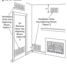
Figure 2 - Ventilation Air from Inside Buildina
